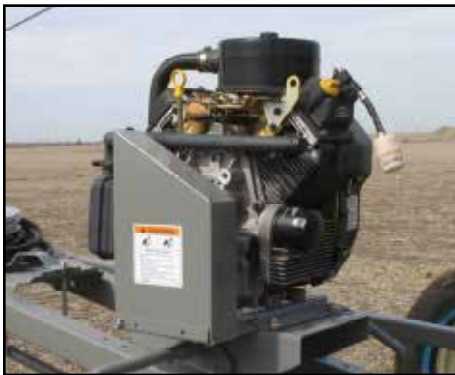
Fig 7 - Engine pulley guard
