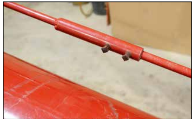
Fig 48 - Set screws to lock rods in place
