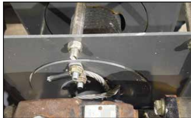
Fig 34 - Winch spool cable retainer
