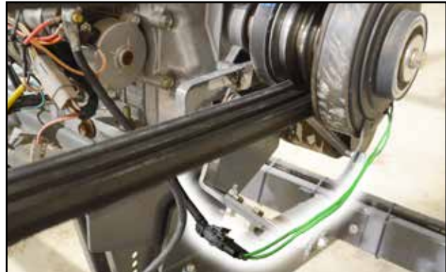
Fig 26 - Clutch wiring harness
