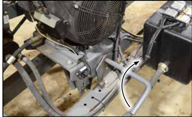
Fig 25 - Engine over-centre cam
