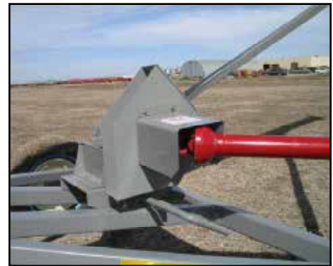
Fig 8 - PTO attachment guard
