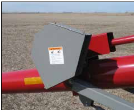
Fig 5 - Gearbox pulley guard
