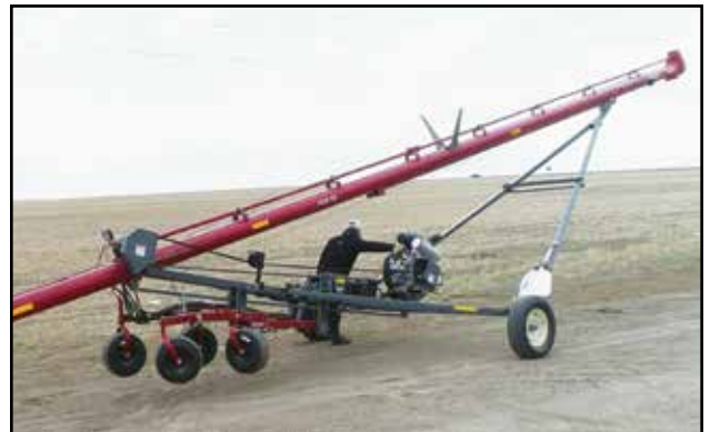
Fig 23 - Auger in transport position
