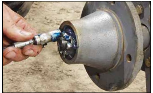
Fig 42 - Fill hub with grease
