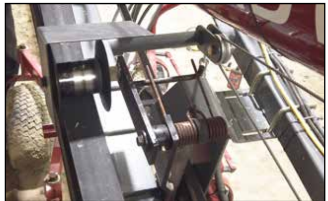
Fig 31 - Spring idler pulley
