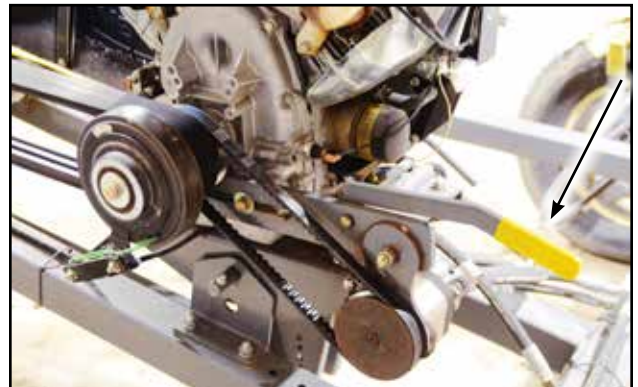
Fig 30 - Pump belt and over-centre cam
