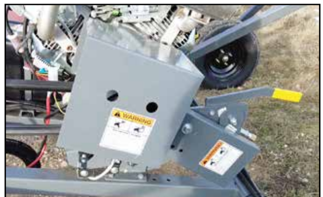
Fig 32 - Clutch and pump belt guards
