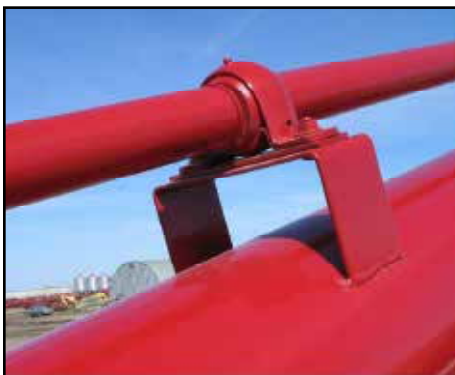
Fig 9 - Tubular drive shaft guard
