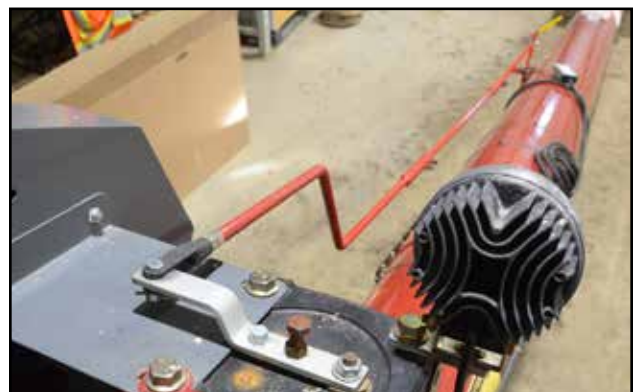
Fig 49 - Rod and linkage installed
