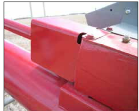
Fig 6 - Gear box shaft guard
