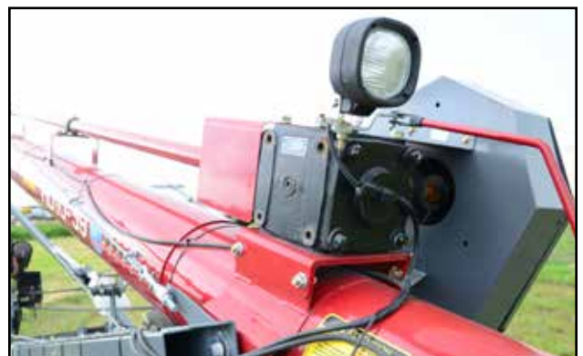
Fig 16 - Gearbox and drive shaft
