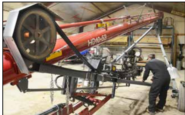
Fig 28 - Open gearbox belt guard
